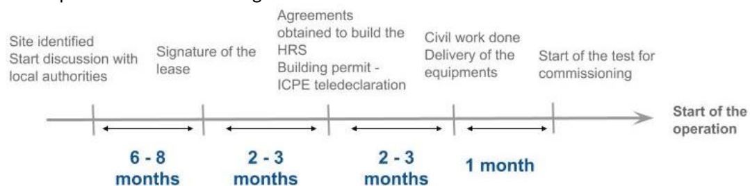
Figure 8 HRS installation process in France (source: Air Liquide)
