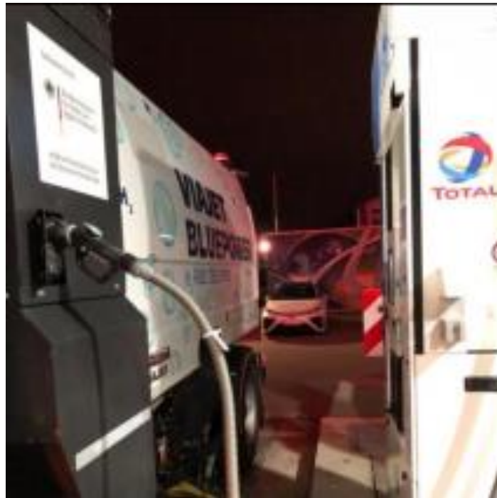
Figure 16: 700 bar refuelling test at Potsdam HRS (source: H2M)
